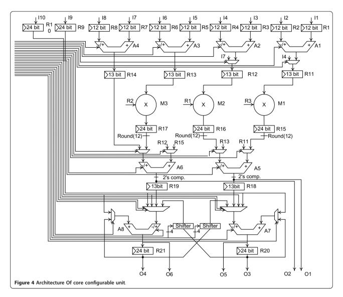
(CACC) operation needs the largest number of simultaneous complex input signals. CACC operation adds or subtracts four complex words every cycle. This puts a constraint on the memory system to supply the unit with a maximum of four words every cycle. However in
