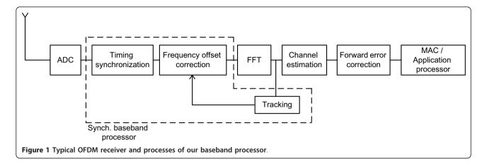
timing offset are performed. To maintain subcarrier orthogonality, CFO is estimated, refined and corrected after determination of frame boundaries. The signal then passes through the FFT block to estimate the transmitted symbols.
